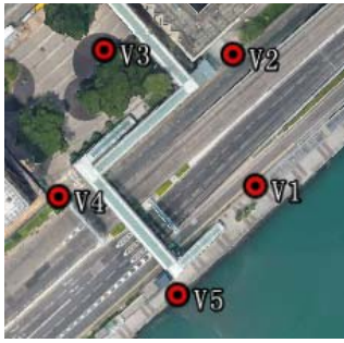
Fig. 7. The selected locations of the five GNSS receivers in the experiment.
